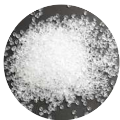
乙烯醋酸乙烯酯共聚合樹脂 Ethylene Vinyl Acetate Copolymer 簡稱 EVA
