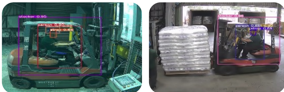
▲ Real-time identification of protective equipment; normal execution determined for the operator
