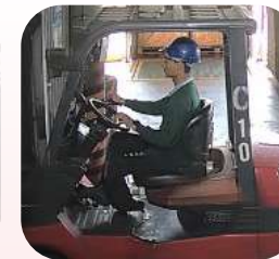
Contractor violations - failure to buckle up helmet strap
