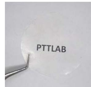
High transparency is maintained on the EVA thin film after adding the nano cellulose.
