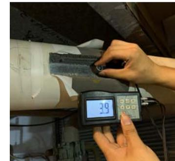
Chiller Water In/Out Temperature Measurement
